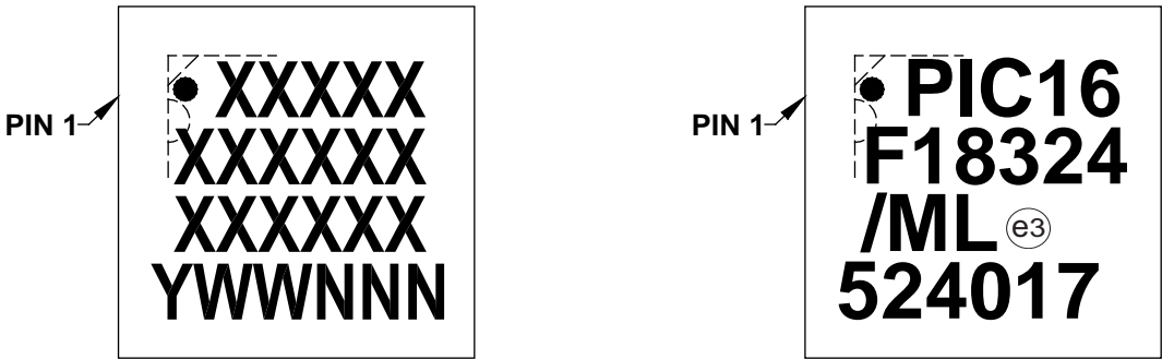
16-Lead UQFN (4x4x0.5 mm)
