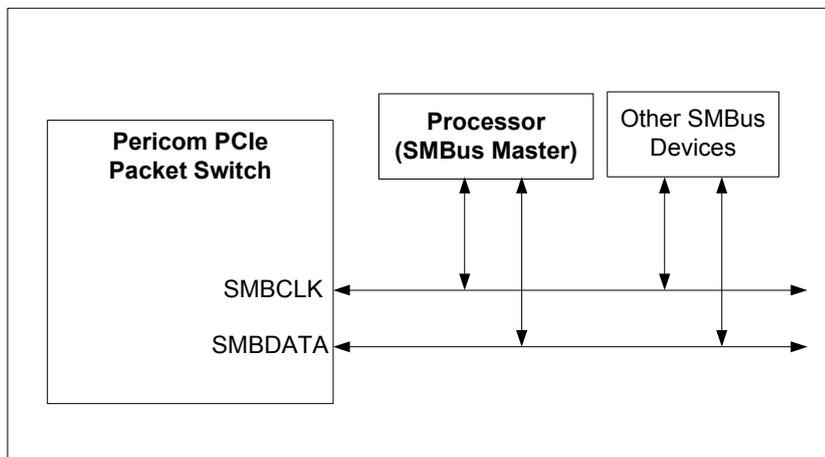
The SMBus interface on the PI7C9X2G404EV consists of one SMBus clock pin (SMBCLK), a SMBus data pin (SMBDATA), and 3 SMBus address pins (GPIO[5:7]). The SMBus clock pin provides or receives the clock signal. The SMBus data pin facilitates the data transmission and reception. Both of the clock and data pins are bi-directional. The SMBus address pins determine the address to which the PI7C9X2G404EV responds to. The SMBus address pins generate addresses according to the following table:
