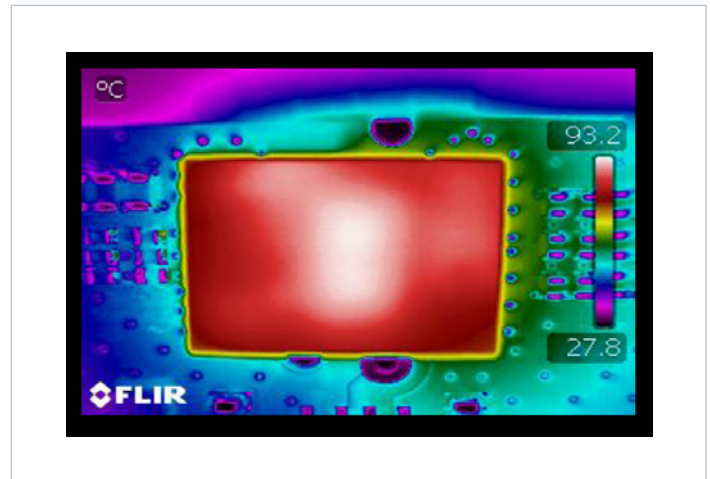
Figure 40 — Thermal Image ( V_{IN} = 28 V, I_{OUT} = 3.33 A, CR, 0 LFM Evaluation PCB)
