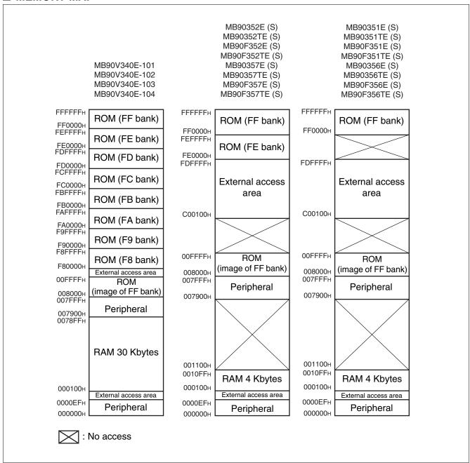
Note: The high-order portion of bank 00 gives the image of the FF bank ROM to make the small model of the C compiler effective. Since the low-order 16 bits are the same, the table in ROM can be referenced without using the far specification in the pointer declaration.
