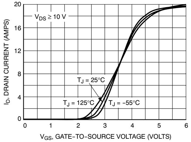
**Figure 2. Transfer Characteristics**
