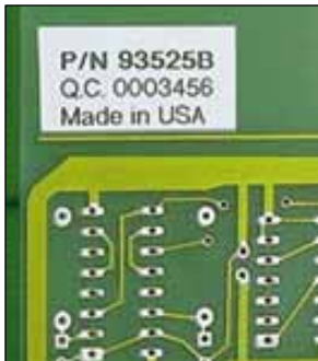
Circuit board labeling
