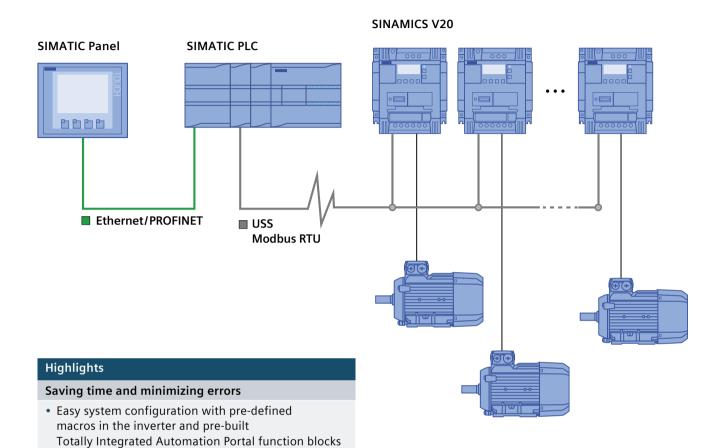
• One cable to connect SINAMICS V20 with USS or Modbus RTU
