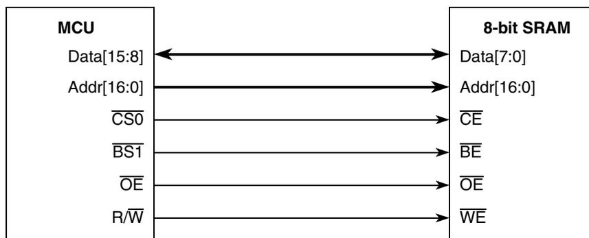
Figure 3-1. 8-bit External SRAM Example
