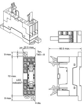
Note 1: The socket is shown with the finger cover removed. 2: Only the -ND Sockets have LED indicators (orange)
