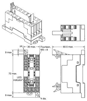
Note 1: The socket is shown with the finger cover removed.
