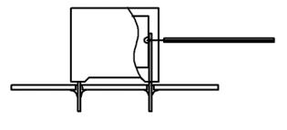
Temperature monitored inside the capacitor.
