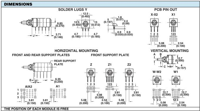
Q В С D Ε F Α **BUSHINGS** DIMENSIONS mm (± 0.5) **DIMENSIONS INCHES (± 0.02)** 0.150 Ε Leads Z00 3.15 1.85 1.85 3.85 0.071 0.071 0.071 0.071 0.071 Leads Z1. Z2. A. 2.8 3.6 Ε 1.6 1.6 0.063 0.063 0.063 0.063 0.063 0.140 Leads Z0.: 5.08 mm (0.200") Leads A.. Z1. Z2.: 3.81 mm (0.150" Leads X.. Y.. 0.200 0.200 0.200 0.278 J 6.7 5 5 0.200 0.200 Leads Z0. with Rotary Switch 0.006 0.0846 Ε 1.45 0.15 0.15 2.15 0.006 0.006 0.006 0.006
