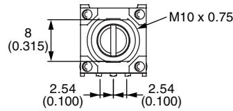
Dual modules, single shaft, PC pins with front support plates, imperial bushing and shaft
