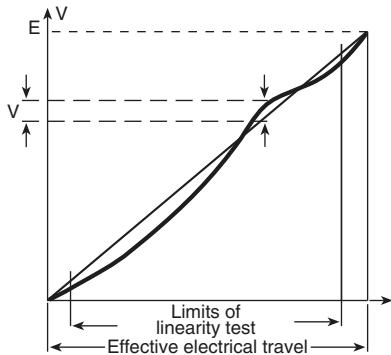
The independent linearity (conformity for the non linear laws) is the maximum gap  $\Delta V$  between the actual variation curve and the theoretical variation curve the nearest to it. The linearity and the conformity are expressed in percentage of the total applied voltage  $E$
