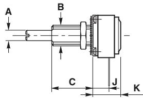
**PANEL AND SHAFT SEALED: BUSHING G**
