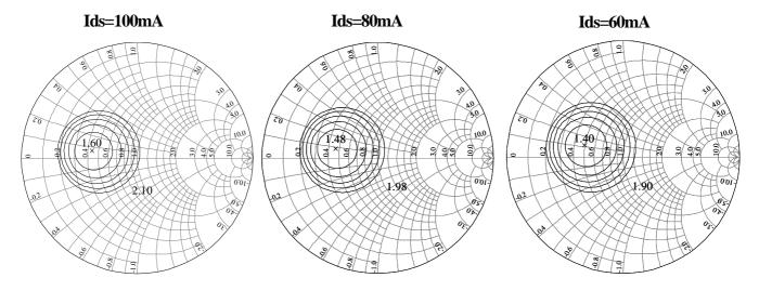
[Note] The data for Smith charts were measured at frequency of 2GHz and Tc of 25°C.
