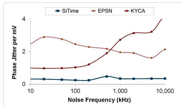
Figure 4. Power Supply Noise Rejection<sup>[4]</sup>
