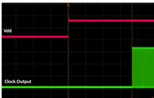
**Figure 18. Startup Waveform vs. Vdd**
