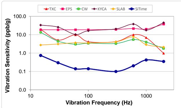
Figure 5. Vibration Robustness<sup>[5]</sup>
