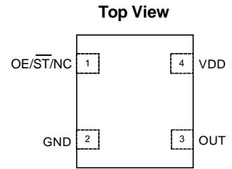
**Figure 1. Pin Assignments**
