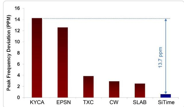
Figure 6. Shock Robustness<sup>[6]</sup>
