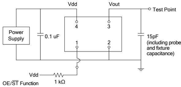
Figure 2. Test Circuit
