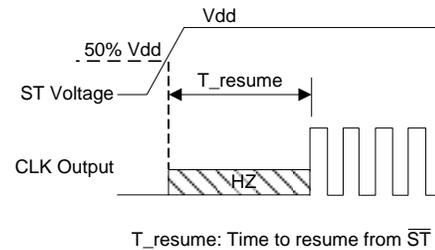
Figure 5. Standby Resume Timing ( $\overline{ST}$  Mode Only)
