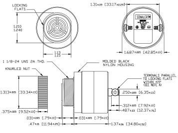
NOTE A: TERMINALS-.032 BRASS TIN PLATED, TAPPED FOR #6-32 SCREW. TWO #6-32 NICKEL PLATED BRASS SCREWS INCLUDED. WILL ACCEPT 1/4\* QUICK CONNECT. NOTE B: MOUNTING- REMOVE BLACK PLASTIC NUT AND INSERT THREADED FRINT THROUGH 1.25' HOLE PUNCHED IN PANEL, IF DRIENTATION IS NEEDED, NOTE LOCKING FLATS ON DRAVING. SCREW NUT BACK ON. DO NOT DVERTIGHTEN.
