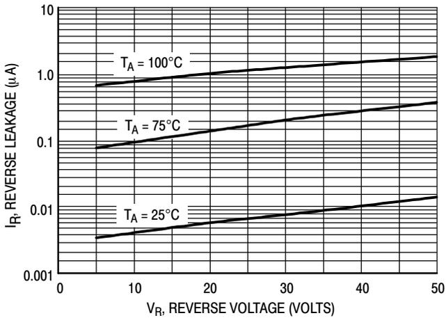
Figure 3. Reverse Leakage
