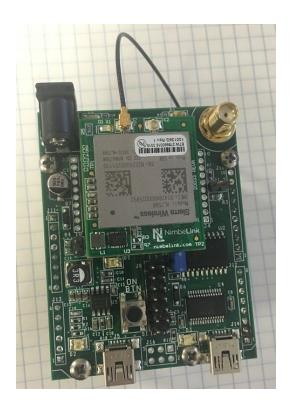
A properly mounted Skywire Modem with U.FL cable attached to top U.FL connector X1
