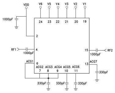
Note: For operations from 700 to 2700 MHz, pins 6 through 13 may be left unconnected.
