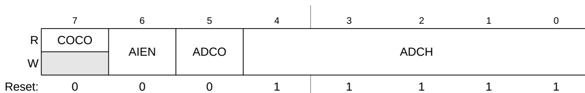
Figure 10-3. Status and Control Register (ADCSC1)
