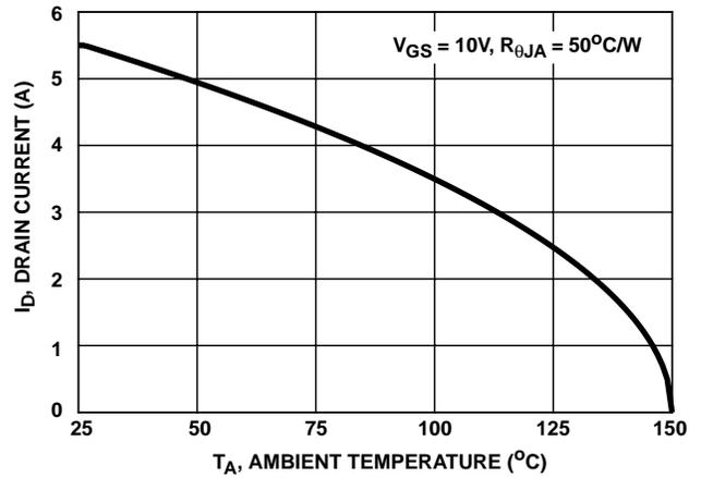
FIGURE 2. MAXIMUM CONTINUOUS DRAIN CURRENT vs AMBIENT TEMPERATURE
