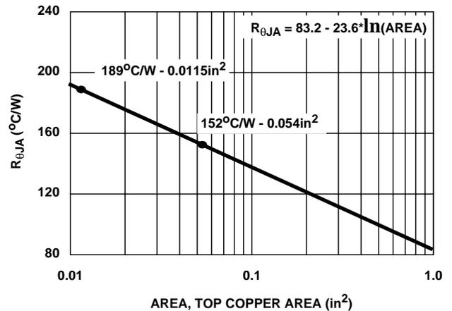
FIGURE 20. THERMAL RESISTANCE vs MOUNTING PAD AREA
