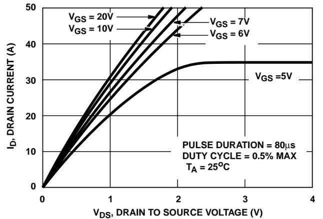
FIGURE 8. SATURATION CHARACTERISTICS
