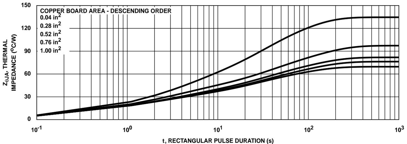
FIGURE 21. THERMAL IMPEDANCE vs MOUNTING PAD AREA
