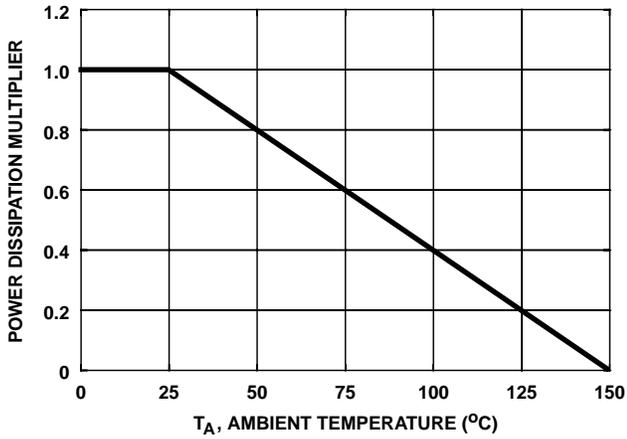
FIGURE 1. NORMALIZED POWER DISSIPATION vs AMBIENT TEMPERATURE
