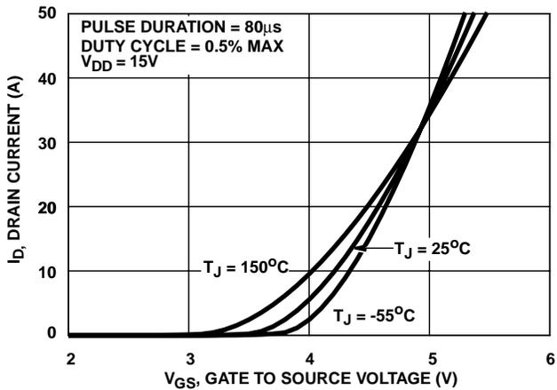
FIGURE 7. TRANSFER CHARACTERISTICS
