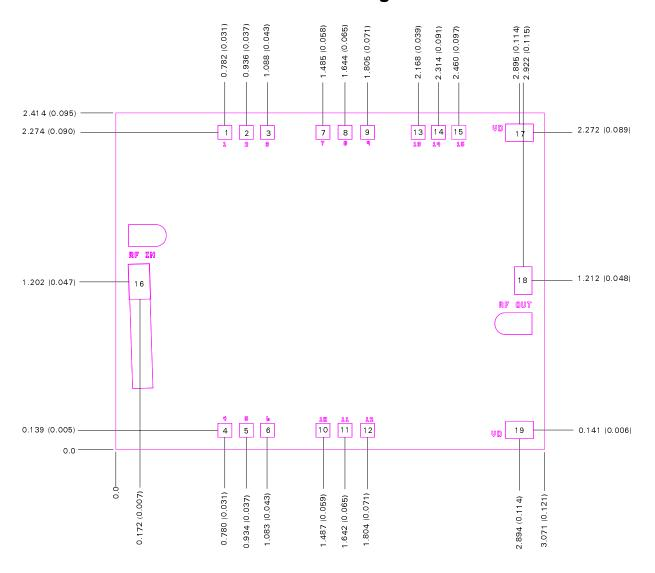
Units: millimeters (inches) Thickness: 0.150 (0.006)
