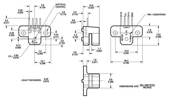
Mounting Option #51 – Screwmount (Baseplane Mounting)
