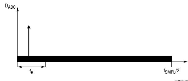
Figure 20. Frequency Spectrum of SAR ADC Core Output
