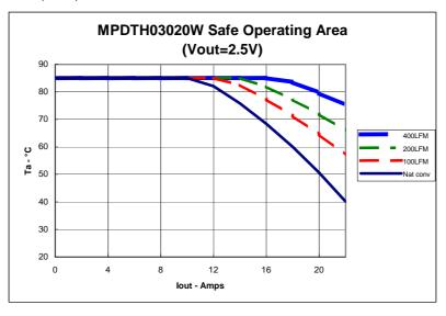
The above SOA represents the condition at which internal components are at or below the manufacturer's maximum operating temperatures. Derating limits apply to modules soldered directly to a 4 in. ×4in. 4-layer PCB with 1 oz. copper. For more reliable operation, appropriate derating is desirable.
