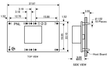
[unit: mm] Tolerance: 0.25mm
