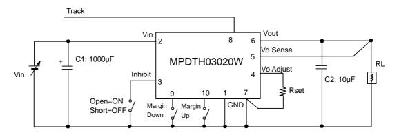
$\begin{array}{lll} \text{C1} & : & 1000 \mu \text{F}/25 \text{V} & (\text{Aluminum Electrolytic Capacitor}) \\ \text{C2} & : & 10 \mu \text{F}/6.3 \text{V} & (\text{Ceramic Capacitor}) \\ \end{array}$
