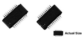
OSOP Series resistor networks feature a space saving 25 mil lead pitch versus the current 50 mil pitch standard. This allows users to reduce board space more than 50 % over current standards. The OSOP series features 16, 20, and 24 pin variations with isolated and last pin common schematics. Custom schematics and resistor values are also available, consult factory.
