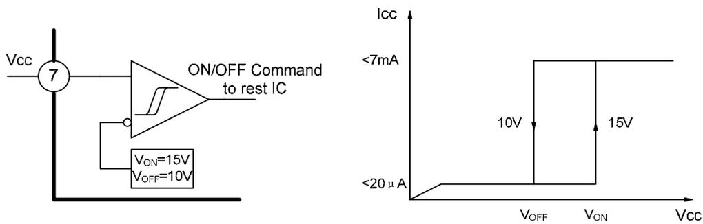
During Under-Voltage Lockout, the output driver is biased to a high impedance state. Pin6 should be shunted to GND with a bleeder resistor to prevent activating the power switch with output leakage currents.
