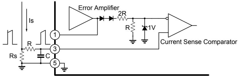
Peak current ( $I_s$ ) determined by the formula:  $I_{S_{MAX}} = 1V/R_s$ . A small RC filter be required to suppress switch transients
