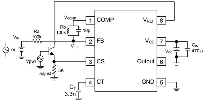
High peak current associated with capacity loads necessitate careful grounding techniques. Timing and bypass capacitors should be connected close to pin5 in single point GND.
