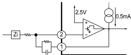
Error amplifier can source or sink up to 0.5mA
