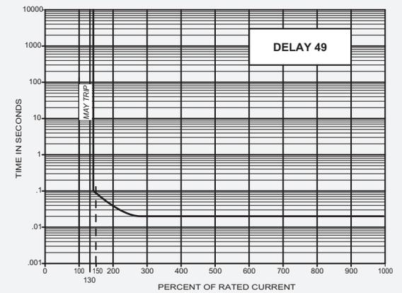
**DC/50/60Hz Dual-frequency Delay Curves (typ)**
