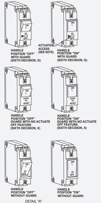
NOTE: ACCESS IS LIMITED TO A DEVICE SMALLER THAN THE UNDERWRITERS LABORATORY "ARTICULATED PROBE" DEFINED IN UL-489 FIG. 11.1.7.2.1.
