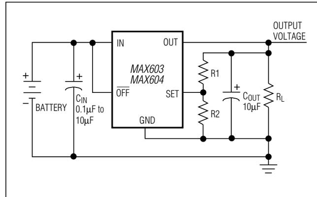
Figure 3. Adjustable Output Using External Feedback Resistors
