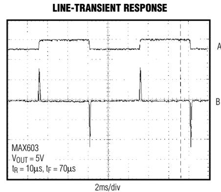
A:  $V_{IN} = 8V$  (HIGH),  $V_{IN} = 7V$  (LOW)
