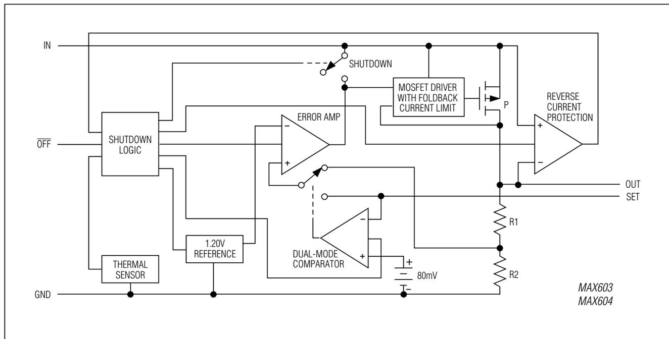
Figure 2. Functional Diagram
