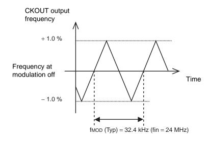
• Modulation rate - 1.0%, example of down spread
