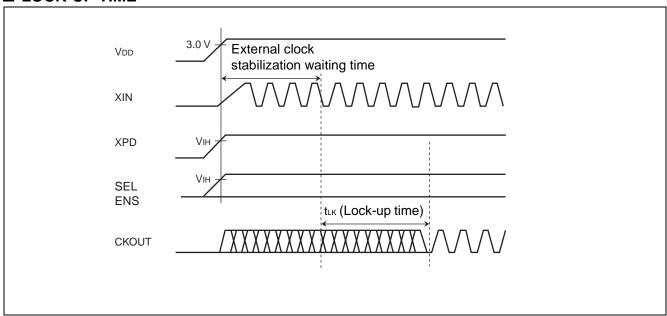
If the XPD pin is fixed at the "H" level, the maximum time after the power is turned on until the set clock signal is output from CKOUT pin is (the stabilization wait time of input clock to XIN pin) + (the lock-up time "tlk"). For the input clock stabilization time, check the characteristics of the resonator or oscillator used.
