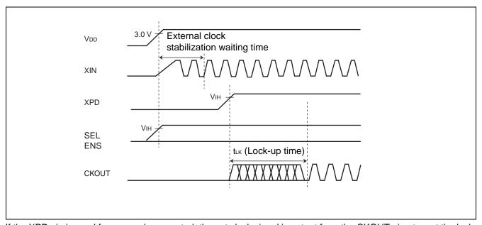
If the XPD pin is used for power-down control, the set clock signal is output from the CKOUT pin at most the lock-up time "tlk" after the XPD pin goes "H" level.
