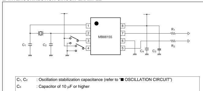
$C_4$ : Capacitor of about 0.01  $\mu F$  (connect a capacitor of good high frequency property
