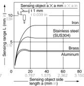
As the sensing object size becomes smaller than the standard size (iron sheet  $30 \times 30 \times t$  1mm  $1.181 \times 1.181 \times t$  0.039 in), the sensing range shortens as shown in the left figure.
