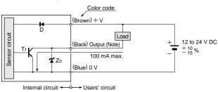
Note: If a capacitive load is directly connected to the output, malfunction may occur.
