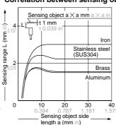
As the sensing object size becomes smaller than the standard size (iron sheet  $12\times12\times t$  1 mm  $0.472\times0.472\times t$  0.039 in), the sensing range shortens as shown in the left figure.
