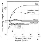
As the sensing object size becomes smaller than the standard size (iron sheet  $70 \times 70 \times t$  1 mm  $2.756 \times 2.756 \times t$  0.039 in), the sensing range shortens as shown in the left figure.
