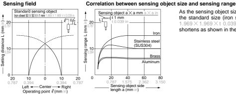
As the sensing object size becomes smaller than the standard size (iron sheet  $50 \times 50 \times t$  1 mm  $1.969 \times 1.969 \times t$  0.039 in), the sensing range shortens as shown in the left figure.
