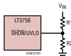
Figure 1. Resistor Connection to Set V<sub>IN</sub> Undervoltage Shutdown Threshold
