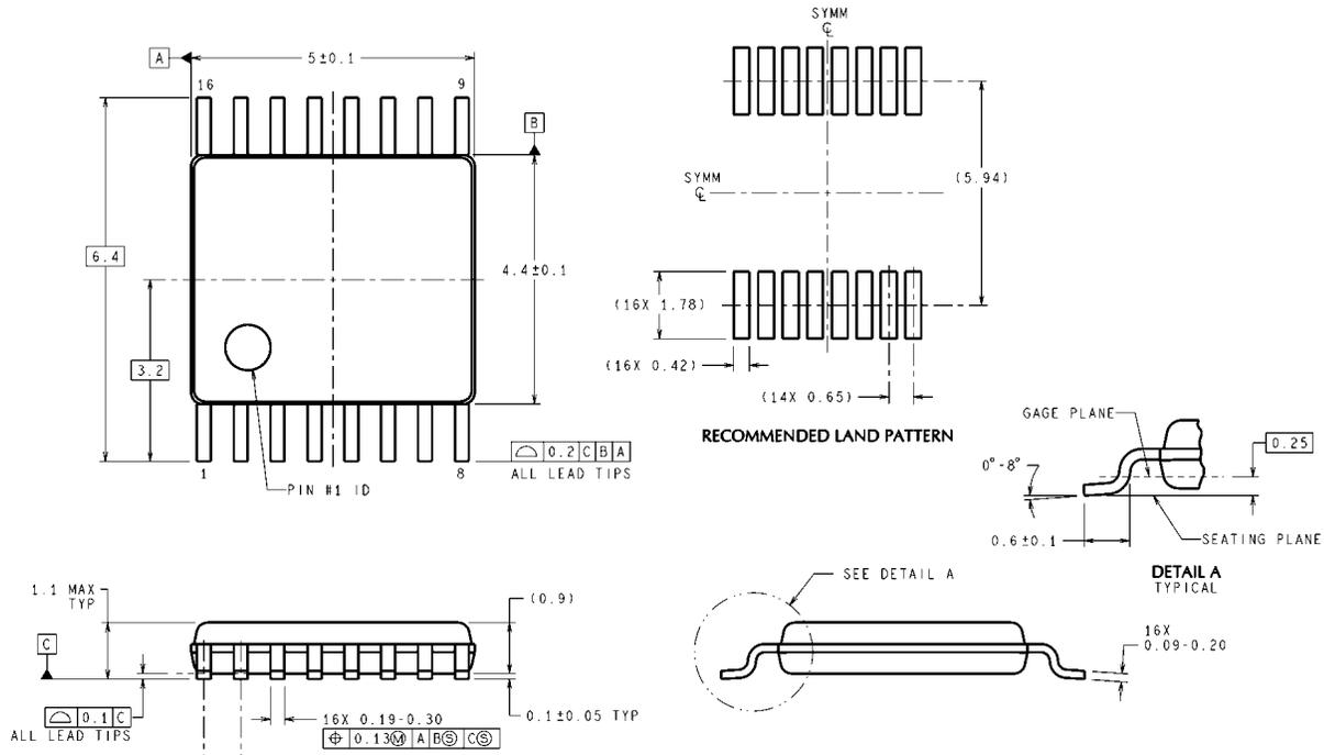
DIMENSIONS ARE IN MILLIMETERS
