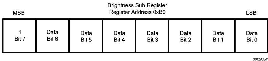
**FIGURE 8. Brightness SUB Register Description**
