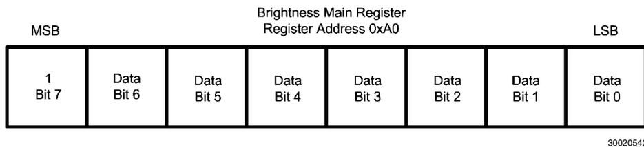
**FIGURE 7. Brightness MAIN Register Description**
