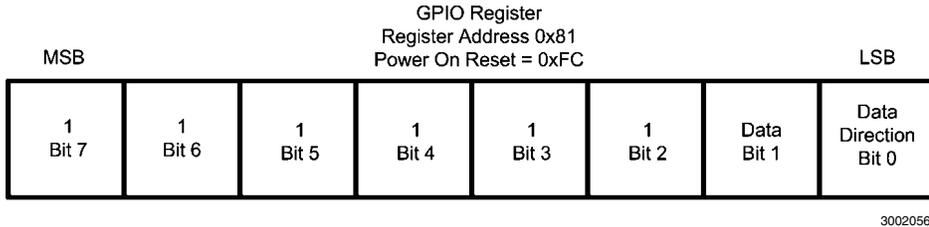
**FIGURE 11. GPIO Register Description**
