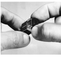
1. Slip mounting clip over top of switch/ indicator housing.
