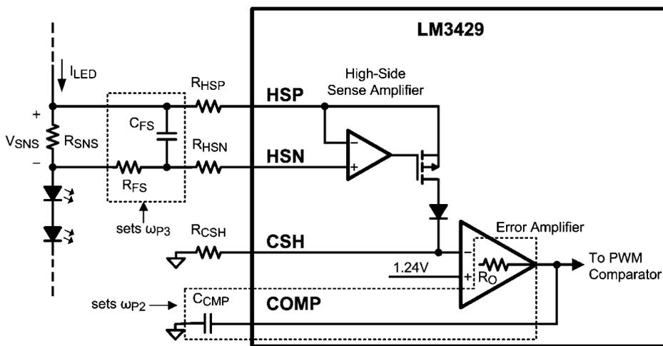
**FIGURE 8. Compensation Circuitry**
