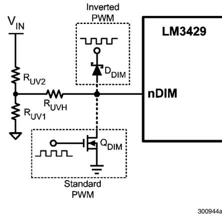
FIGURE 13. PWM Dimming Circuit
