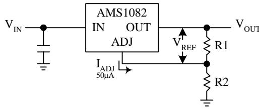
$$V_{OUT} = V_{REF}(1 + R2/R1) + I_{ADJ}R2$$
