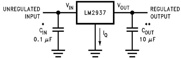
\* Required if the regulator is located more than 3 inches from the power supply filter capacitors.
