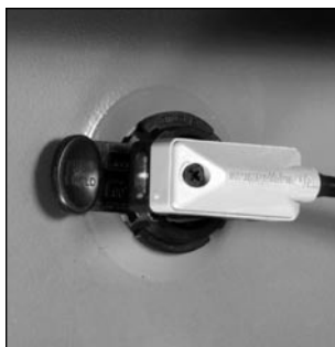
2. Insert the sensor into the bracket as shown.
