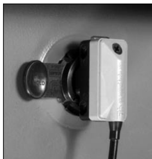
3. Holding the bracket by the tab, rotate the sensor 90° clockwise.
