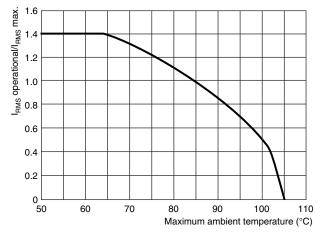
Maximum I<sub>RMS</sub> current in function of the ambient temperature
