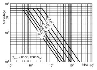
Max. RMS voltage as function of frequency (2000 V)
