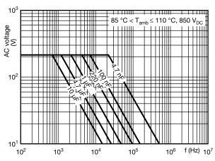
Max. RMS voltage as function of frequency (850 V)
