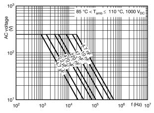
Max. RMS voltage as function of frequency (1000 V)
