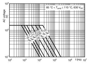
Max. RMS voltage as function of frequency (630 V)
