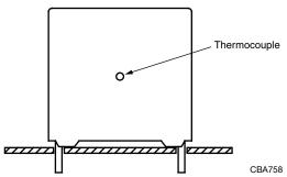
The temperature is measured in unloaded ( $T_{amb}$ ) and maximum loaded condition ( $T_{C}$ ). The temperature rise is given by  $\Delta T = T_{C} - T_{amb}$ .
