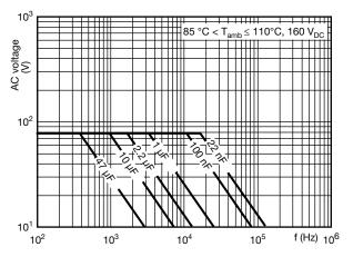
Max. RMS voltage as function of frequency (160 V)
