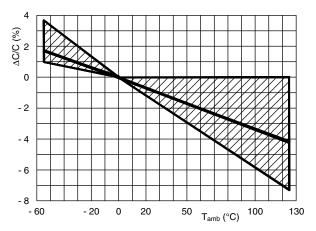
Capacitance as a function of ambient temperature (typical curve) (1 kHz)
