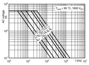
Max. RMS voltage as function of frequency (1600 V)
