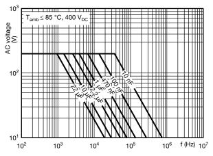
Max. RMS voltage as function of frequency (400 V)
