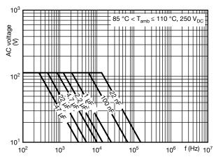
Max. RMS voltage as function of frequency (250 V)
