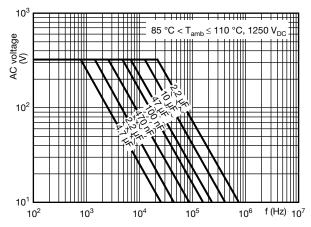
Max. RMS voltage as function of frequency (1250 V)
