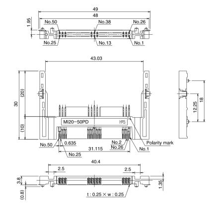
Note 1: Coplanarity of all surface mount terminals and components is 0.1.
