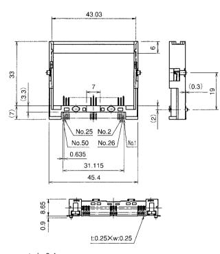
Note 1: Coplanarity of all surface mount terminals and components is 0.1.
