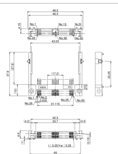
Note 1: Coplanarity of all surface mount terminals and components is 0.1.
