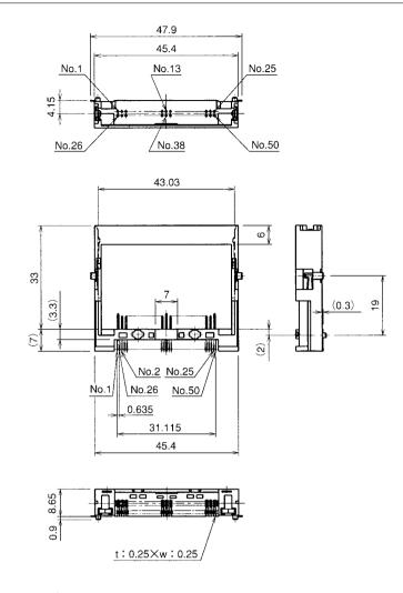
Note 1: Coplanarity of all surface mount terminals and components is 0.1.
