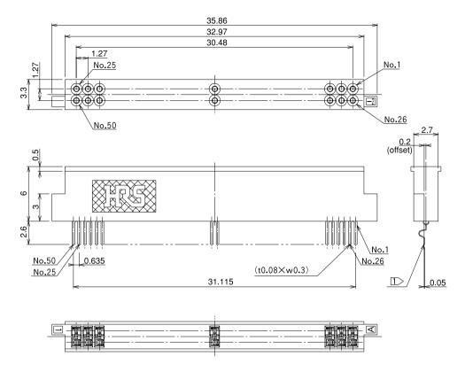
Note 1 The coplanarity of the conductor is 0.1 mm Max.
