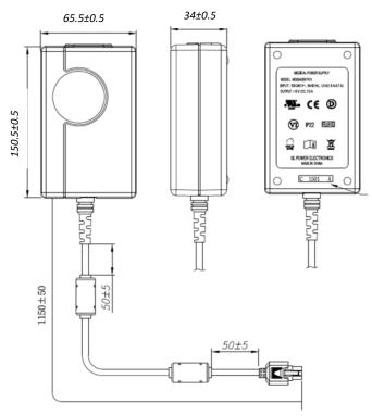
12V Models: Output Connector: 6 pin Molex 39-01-2060 or equiv. Pins 1, 4 = (+), pins 3, 6 = (-), pins 2, 5 = NC
