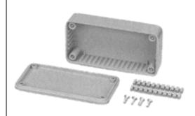
High quality, multipurpose ABS boxes available in a range of sizes. The boxes can be readily drilled and can withstand temperatures of up to 85°C. All sizes incorporate slots on four internal faces for vertically mounting 1.5mm thick PCBs, and are supplied with slotted adapter bars, which allow horizontal mounting. The close fitting, flanged lids are secured by screws (supplied) running into threaded bushes in the base.
