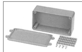
As above but with mounting lugs moulded into the lid. The lugs accept M3 countersunk screws, and allow the box to be mounted on to a wall or panel with the lid retaining screws hidden for limited tamperproofing.
