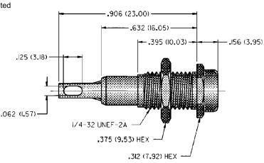
For Standard Tip Plug: .080 (2.00) Diameter FEATURES:
