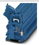
Disconnect terminal block, Connection type: Screw connection, Cross section: 0.14 mm² - 6 mm², AWG: 26 - 10, Nominal current: 20 A, Nominal voltage: 500 V, Length: 57.8 mm, Width: 6.2 mm, Color: blue, Assembly: NS 35/7,5, NS 35/15
