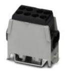
Trunk line branch terminal, Connection method: Screw connection, Number of positions: 1, Cross section: 1.5 mm² - 25 mm², AWG: 8 - 2, Width: 23 mm, Color: black, Mounting type: NS 35/7,5, NS 35/15
