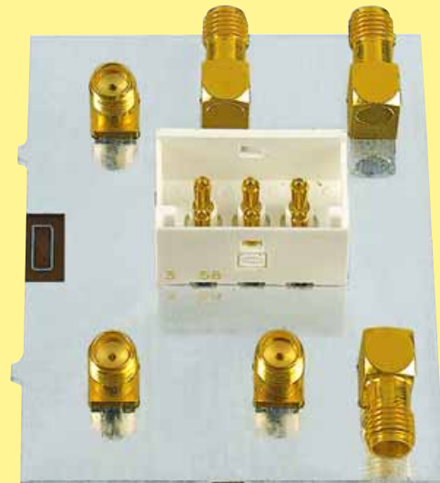
Fig. 6: Test boards with implemented Mini Coax connector
