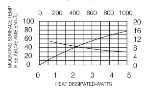
THERMAL RESISTANCE FROM MTG SURFACE TO AMBIENT-C/WATT
