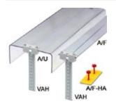
Flat-ribbon cover, for covering terminal strips, 2 mm thick, 6 cm wide, an additional requirement are 2 E/UK end brackets and 2 adjustable VAH cover holders. The max. supply length is 100 cm
