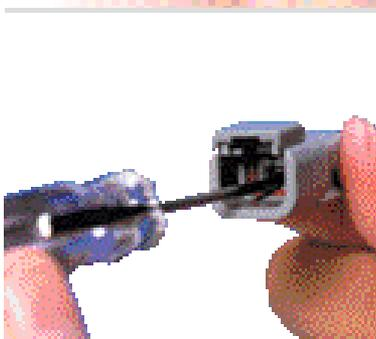
2. To remove the contacts, gently pull wire backwards, while at the same time releasing the locking finger by moving it away from the contact with a screwdriver.
