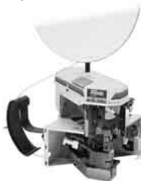
AMP-O-LECTRIC Model "G" Terminating Machine
